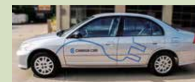
CMU's Robotics Institute's CREATE Lab has developed the "ChargeCar," a battery-powered commuter (short-range) vehicle — stripped of its internal combustion engine, radiator and cooling system, fuel tank, and exhaust system. With the goal of licensing the technology for third-party commercial production, scientists in the Institute for Energy Innovation will study the consumer market for the car and its life cycle and the recharging infrastructure needed to make its use widespread (left).
