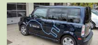
CMU's Robotics Institute's CREATE Lab has developed the "ChargeCar," a battery-powered commuter (short-range) vehicle — stripped of its internal combustion engine, radiator and cooling system, fuel tank, and exhaust system. With the goal of licensing the technology for third-party commercial production, scientists in the Institute for Energy Innovation will study the consumer market for the car and its life cycle and the recharging infrastructure needed to make its use widespread (left).
