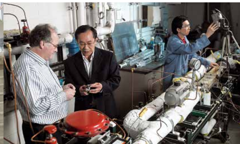
Pitt's Center for Energy researches ways to improve the thermal efficiency of advanced turbine systems in order to enable turbine blades inside large generators to operate at higher temperatures with greater resiliency and improved power generation. Shown (left to right) are Center for Energy Director and Professor of Advanced Turbine Technologies Brian Gleeson and Minking Chyu, Chair of the Department of Mechanical Engineering and Materials Science, and postdoctoral student Sin Chien Siw.
