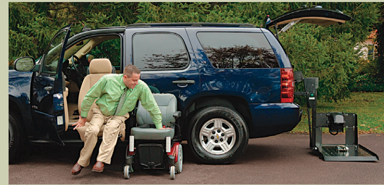
Freedom Sciences, LLC integrates advanced robotics technology with existing mobility devices into a cost-effective solution for independent transportation mobility. Its product includes a platform lift and dock, an articulating automotive seat, and the robotics for remote control of a power wheelchair.
