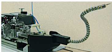
Cardiorobotics' cardioARM™ is intended to provide multiple applications for a wide range of epicardial interventions through a single incision below the rib cage as opposed to open heart surgery. The company expects to begin human clinical trials in 2010.
