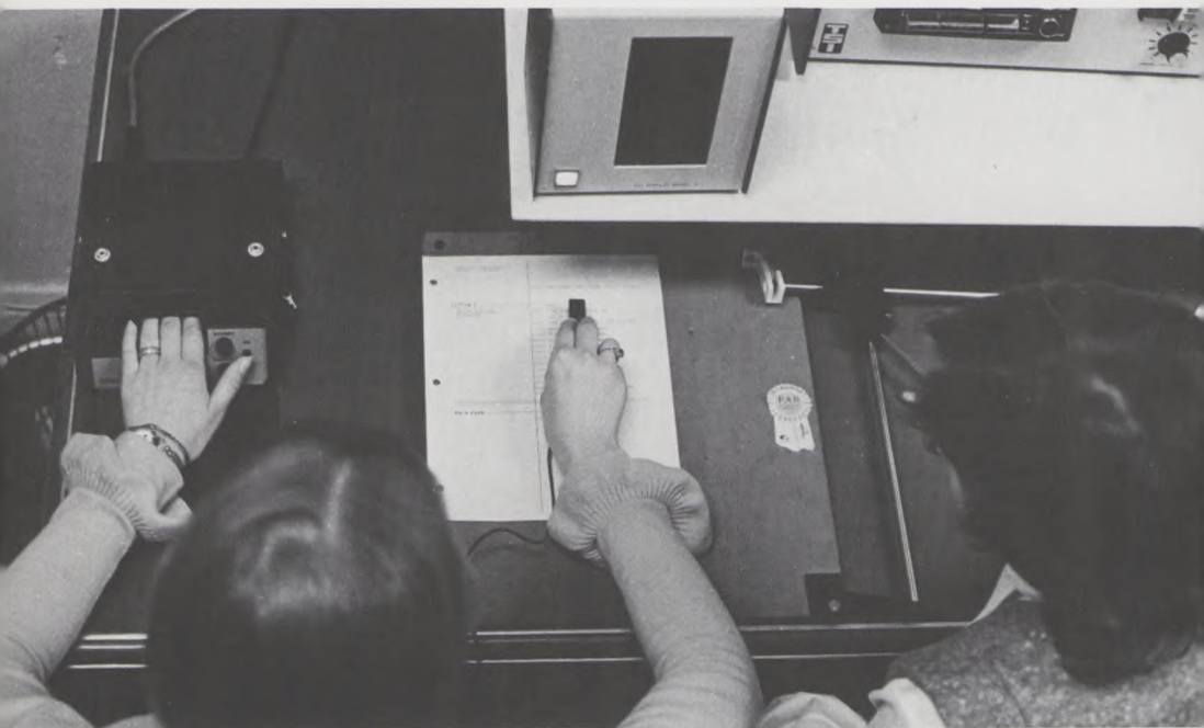
Optacon training at the Pittsburgh Branch, Pennsylvania Association for the Blind. The trainee, left, scans printed material with tiny camera held in her right hand, while simultaneously feeling
